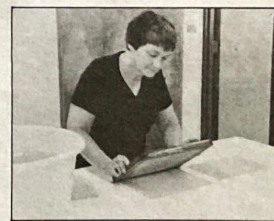
Lifting screen from paper sheet to begin drying process.
