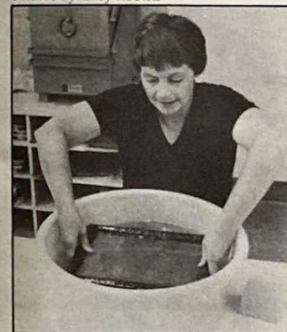
Dipping screen into vat of suspended pulp.
