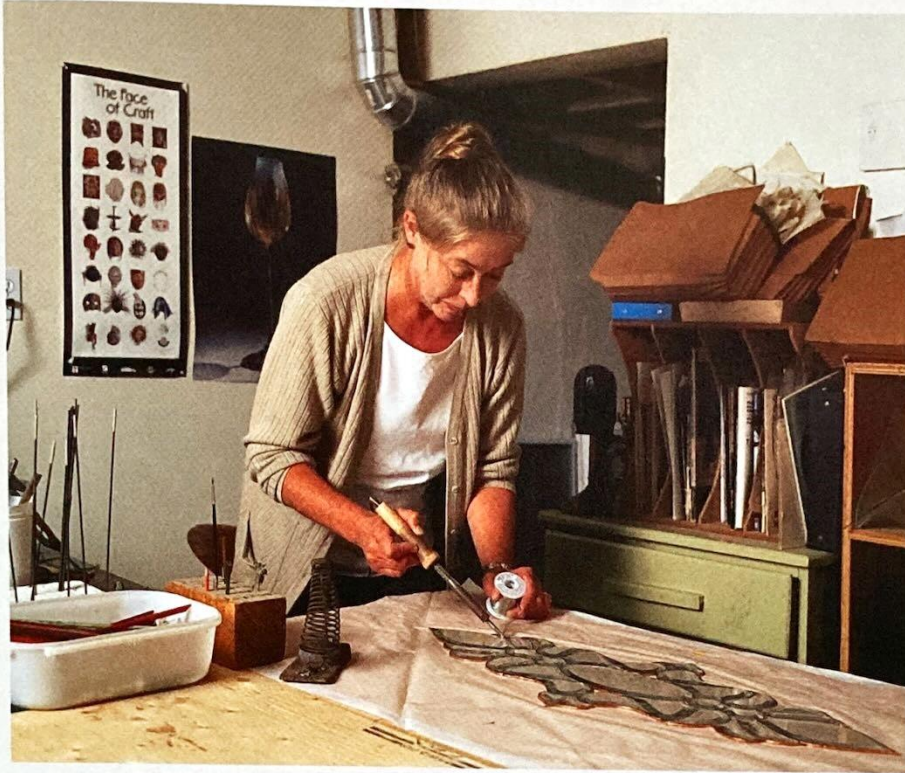
Linda Forbes assembling the bevel cluster before the perimeter glass is soldered on.
