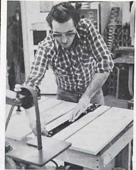
Marking out guitar necks with template.
