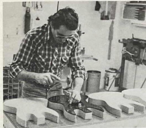
Marking out screw holes with template.
