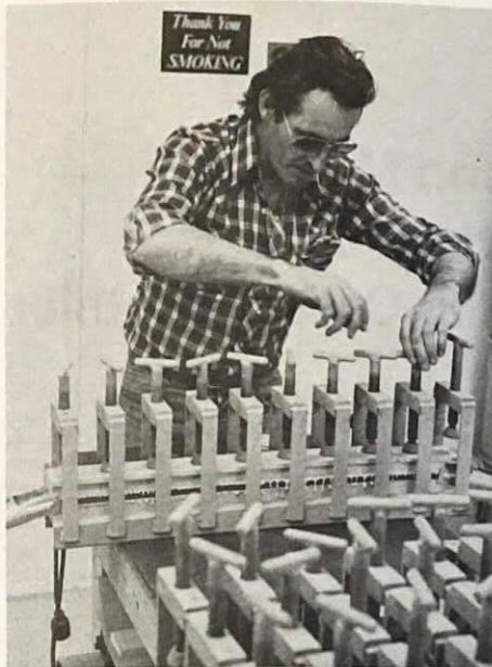
Gluing neck blanks with McDougall-designed clamps.
