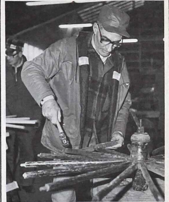
Seating a spoke into a hub. Jack Shepherd, Maple Creek. (Photos by R. Izumi, courtesy the Western Development Museums)
