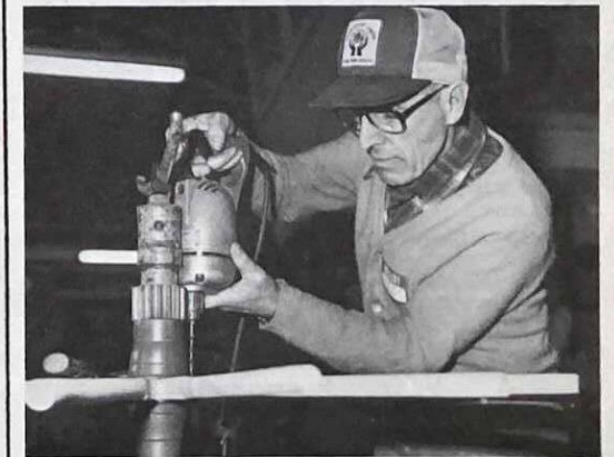
Drilling a rivet hole in a spoke. Ernie Ford, Humboldt.
