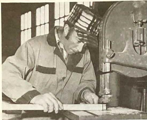
Band sawing the tongue on a spoke. Ray Ostrom, Biggar and District Museum.
