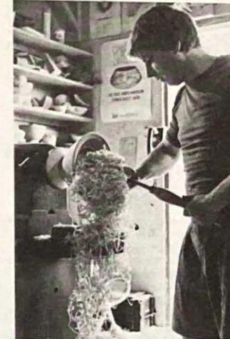
Shavings flow out of a bowl as wood is cut with a gouge.
